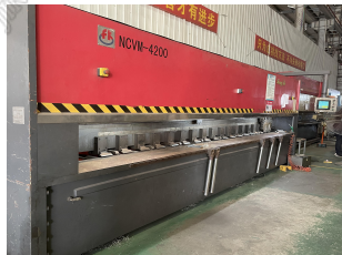
V groove planning equipment 刨槽机
