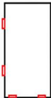
1. FIXED FLOOR AND LEFT SIDE OF THE WALL.
